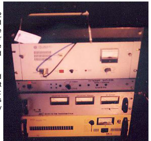
Above : The collection of equipment atop the Space Probe in 1997. The 1RU unit is a gain block to match the MPX output of the RL900 to the input of the CTE. The squelch circuit on the RL900 was modified, so as to switch the equipment on and off whenever a carrier was detected from the Greenhouse, usually about 10:30pm every Friday night.
