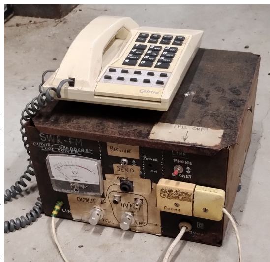
Below : Outside Broadcast Line Driver, as used with Crossbar Links in the 1990s. Lower photo shows inside.
